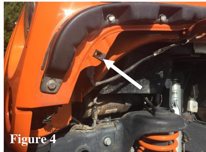
Step 7 – Install the supplied 5/16”-18 button head screw that is closest to the grille into the 5/16”-18 clip nut you previously installed in Step 5.
