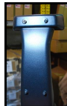
Remove Brake Light Back Cover
